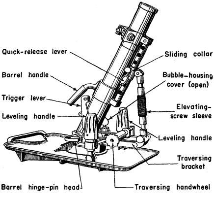
Figure 53.—Right side of 5-cm mortar.
