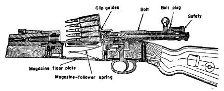
Figure 12.—Cross section of magazine, trigger, and bolt mechanism of Mauser Kar. 98K rifle.
