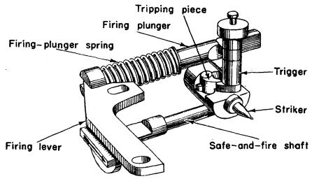
Figure 83.—Firing mechanism of 10.5-cm light field howitzer 18 (1.F.H. 18). (This firing mechanism is similar to that of the 15-cm infantry howitzer.)
