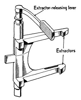
Figure 68.—Extractors of 5-cm Pak.
