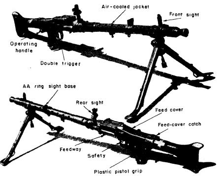
Figure 33.-Two views of M.G. 34 on bipod mount.
