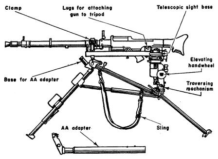
Figure 35.—M.G. 34 on tripod mount, and with antiaircraft adapter.
