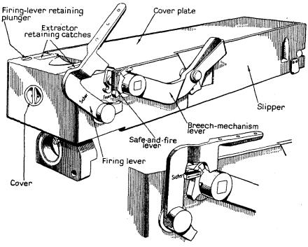
Figure 73.—Breechblock and firing mechanism of 7.5-cm infantry howitzer.
