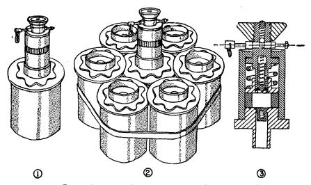
Figure 30.—(1) Stick grenade antipersonnel mine. (This mine is improvised from the head of a stick grenade and pressure igniter 35 (Druckzünder 35, D.Z. 35), which is screwed into the head of the grenade.)
