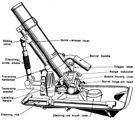
Figure 52.—Left side of 5-cm mortar.
