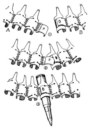
Figure 47.—Method of joining metallic-link ammunition belt.
