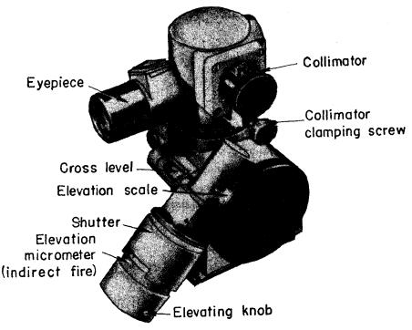
Figure 44.—Telescopic sight for M.G. 34 (rear view).
