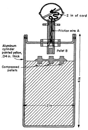
Figure 28.—Cross section of shaving-stick grenade.
