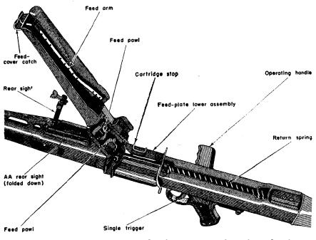
Figure 50.—M.G. 42 with feed cover raised to show feed mechanism.
