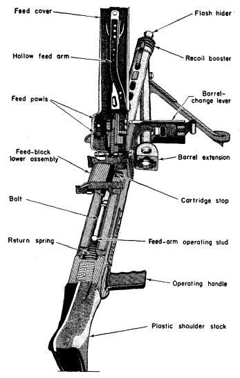
Figure 51.—M.G. 42, showing method of operating barrel extension.
