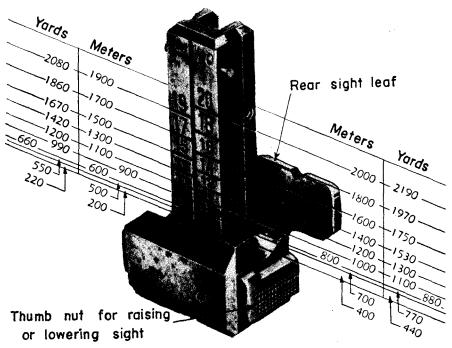
Figure 42.—Rear sight of M.G. 34, showing relation between yards and meters.
