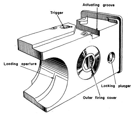
Figure 85.—Breechblock (rear view) of 10.5-cm light field howitzer (1.F.H. 18).
