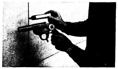
Figure 17.—Pistol grenade being breech-loaded.
