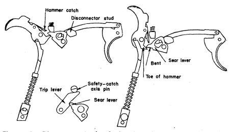
Figure 7.—Diagrammatic sketch showing trigger action of Walther pistol.
