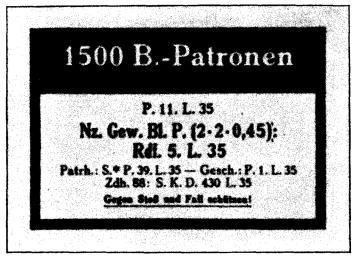
Figure 98.—Label for 1,500 rounds of observation (explosive) bullets (B.-Patronen, Beobachtungsgeschoss Patronen). (This label is white with black printing. The underlined printing is a caution: Protect against shock and dropping!)
