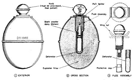
Figure 27.—Sketch of Eierhandgranate 39 (egg-type hand grenade, model 39).
