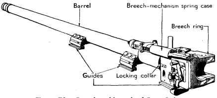
Figure 70.—Barrel and breech of 5-cm Pak.
