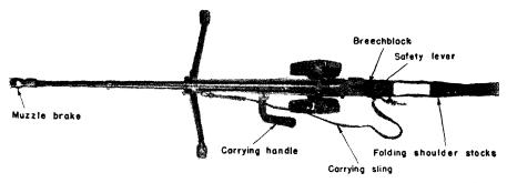
Figure 22.—Overhead view of Pz.B. 39, illustrating cutout folding shoulder stock.
