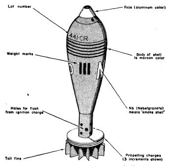
Figure 115.—8-cm mortar shell.
