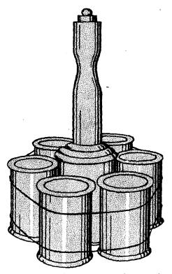
Figure 29.—Concentrated charge (geballte Ladung) made from several stick grenades. (This charge is used for demolition purposes.)
