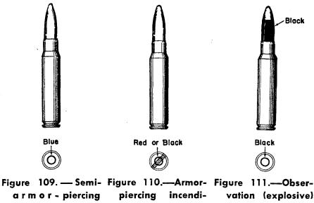
ermor - piercing (Patronen Spitzgeschoss mit Eisenkern). gure 110.—Armorpiercing incendiary (Patronen Phospor mit Stahlkern). (The bullet is black or red in the primer seat, or has a red band across the base.) gure 111.—Observation (explosive) bullet (Beobachtungsgeschoss Patronen). (The bullet is black except for the tip; early issues have chromimum - plated tip only.)
