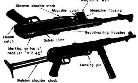
Figure 8.—Two views of M.P. 40, showing skeleton shoulder stock folded, and open.
