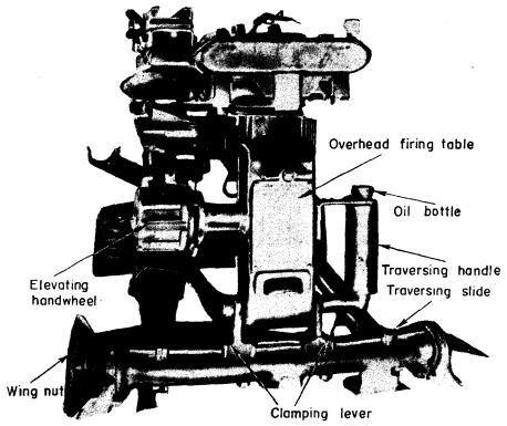
Figure 46.—Rear view of tripod mount for M.G. 34. (See tables 1 and 2, pp. 76–77, below, for a translation of the plate containing overhead firing data.)
