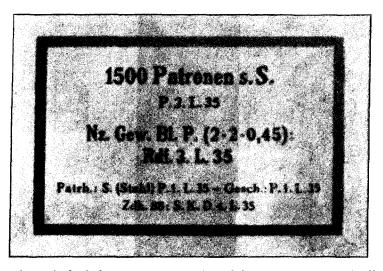
Figure 96.—Label for 1,500 rounds of heavy, pointed ball ammunition (Patr. s. S., Patronen schweres Spitzgeschoss). (The label is white with black printing. A vertical blue band runs through the center, indicating the cartridge cases are steel instead of brass; notice also the word Stahl ("steel").)
