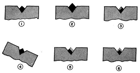
Figure 5.—Method of using German sights. (1) illustrates correct sight picture; 2), firing high; 3), low and right; 4), low and right; 5), lower left; 6), low shot.)
