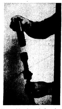
Figure 14.—Grenade launcher, showing method of unscrewing it to aid in cleaning.
