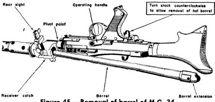
Figure 45.—Removal of barrel of M.G. 34
