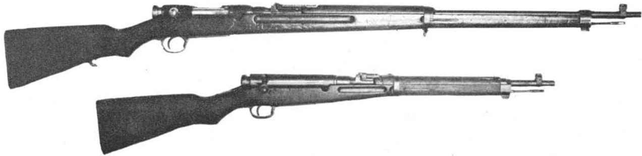
Figure 36. Japanese rifles: Model 38 (1905) 6.5-mm rifle (above) and Model 38 (1905) 6.5-mm carbine.
