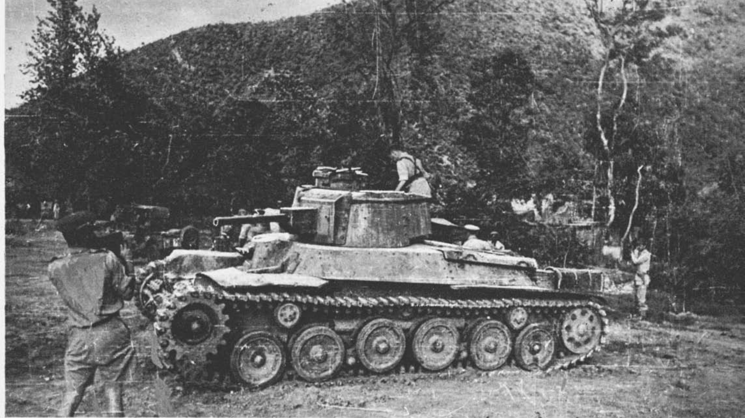
Figure 93-B. Model 97 (1937) medium tank with 47-mm gun.
