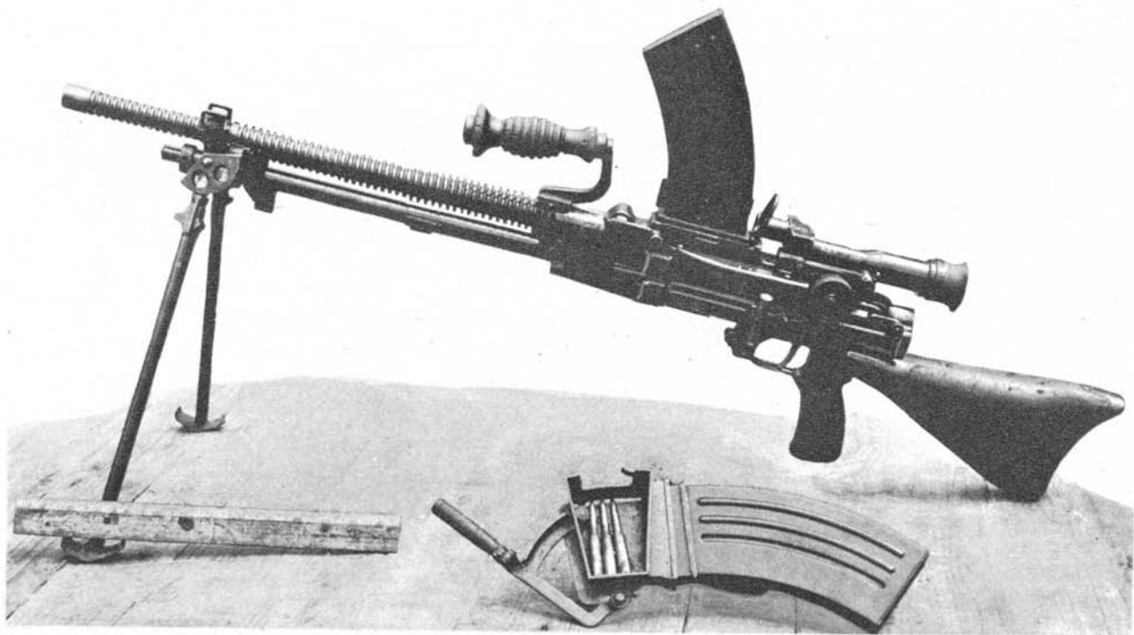
Figure 55. Model 96 (1936) 6.5-mm light machine gun.
