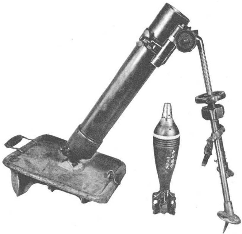
Figure 65. Model 99 (1939) 81-mm mortar.
