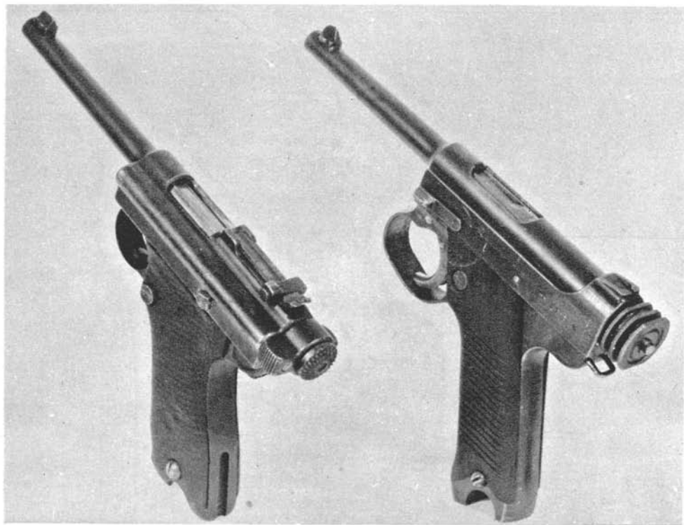
Figure 34. Nambu and Model 14 8-mm pistols.
