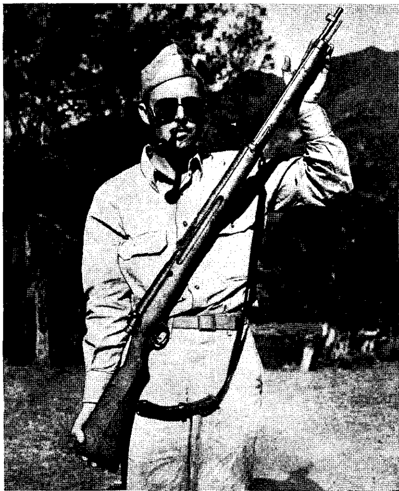
Figure 17.—Model 38 (1905) 6.5-mm rifle, showing its unusual length.
