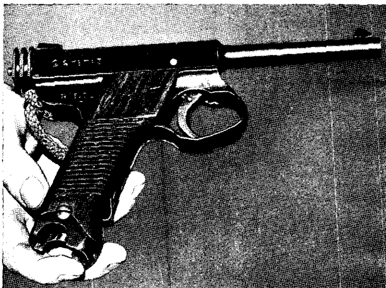
Figure 11.—Model 14 (1925) 8-mm pistol (right side), showing lanyard.
