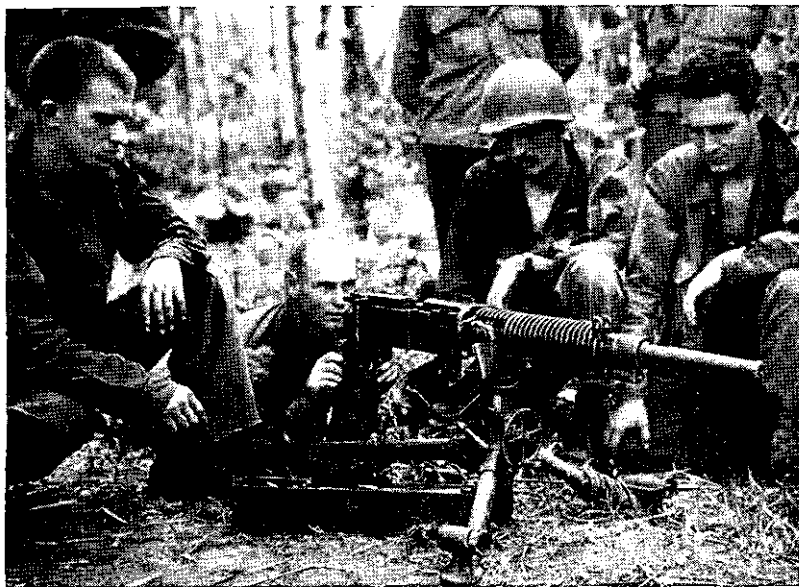
Figure 77.—Model 92 (1932) 7.7-mm heavy machine gun, showing tool and spare-parts box.
