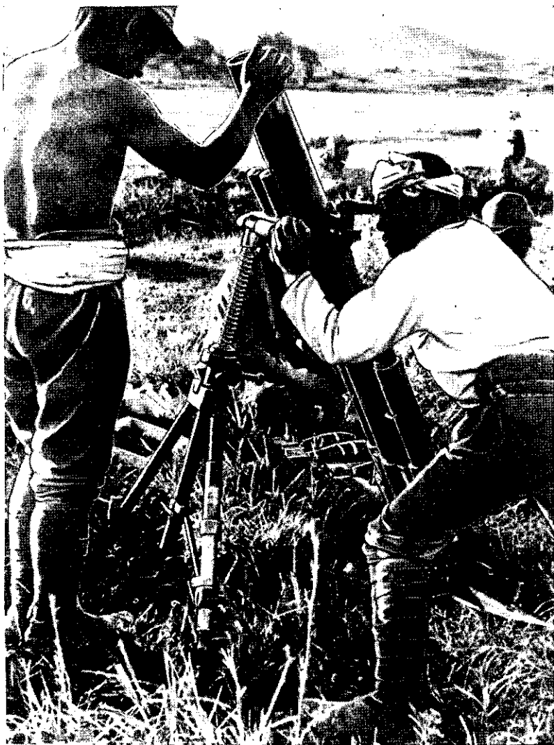
Figure 99.—Laying-in Model 94 (1934) 90-mm mortar.
