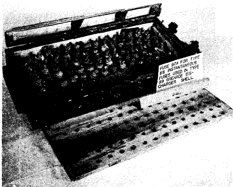
Figure 52.—Packing box for fuzes used in Model 89 (1929) 50-mm shells (100 fuzes).
