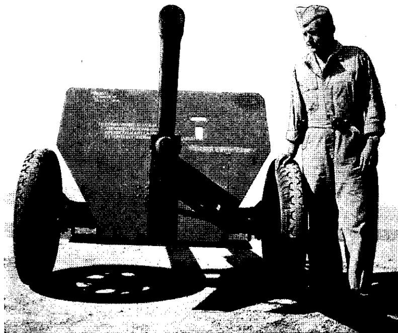
Figure 134.—Model 1 (1941) 47-mm gun (front view).
